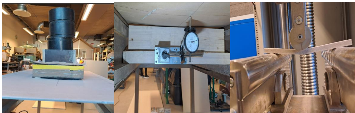
Fig. 1. Setup of the experiment: left – view from the top; middle – view from the bottom; right – three-point bending test setup on a Zwick/Roell Z600
